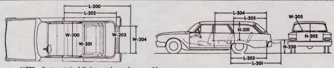
NOTE: Front seat in full down and normal rear position for all measurements. Lengths and heights measured at car centerline.
